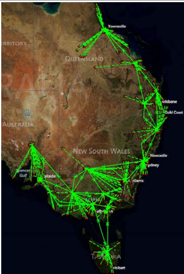
In the September-October 2012 newsletter we described work in the Future Grid Forum . Above is a schematic of an expanded interconnected grid on Australia's East coast, consisting in this case of 509 generation plants and 40 main interconnectors between regions. Both Gurobi and CPLEX are being used to solve generation and transmission design MIP problems as part of the FGF work, in tandem with energy market simulators.
