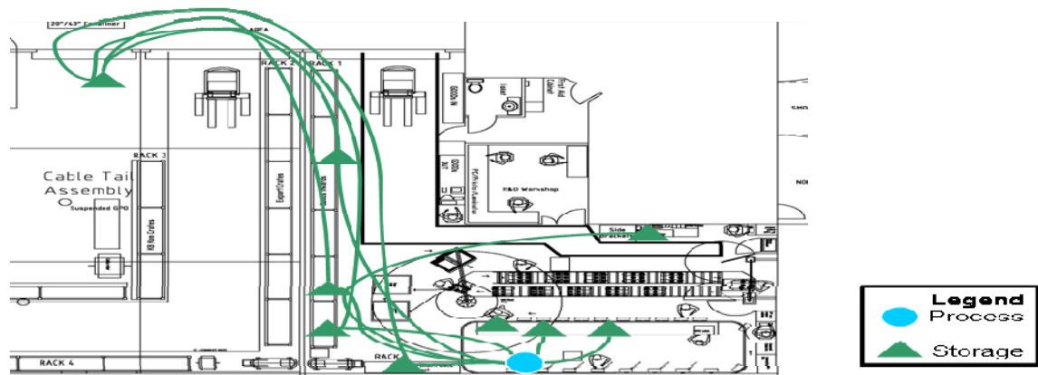
Figure 4: RC cubicle assembly material flow
